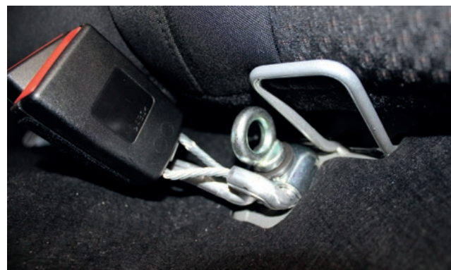
Multimac eye bolt replaces original bolt
