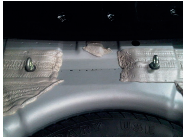
Floor drilled and eye bolts fitted
