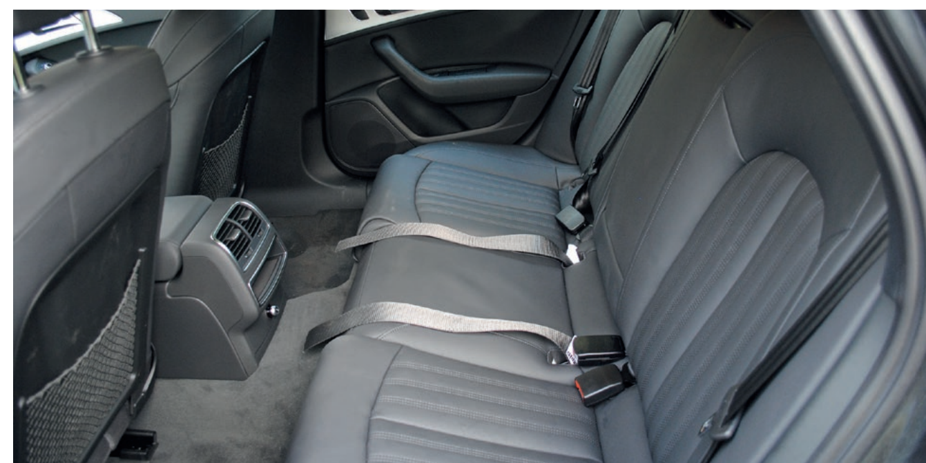
Seat cushion refitted: replacement buckles fed through the gap behind the cushion, tether straps fed through the original buckle holes
