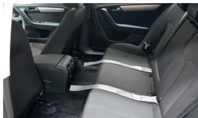
Cushion replaced, showing tether straps and buckles both fitted
