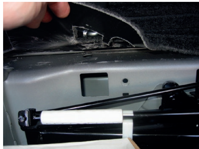
Existing holes in Range Rover [L322] used for fitting eye bolts and spreader plates and showing tether straps fitted
