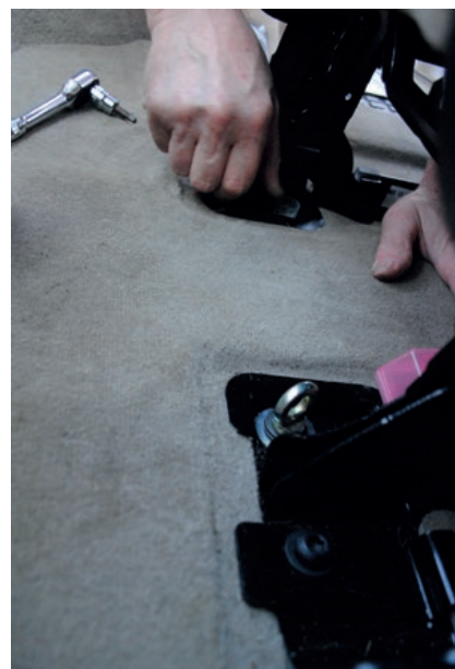
Examples showing eye bolt fixings, and tether strap routings
