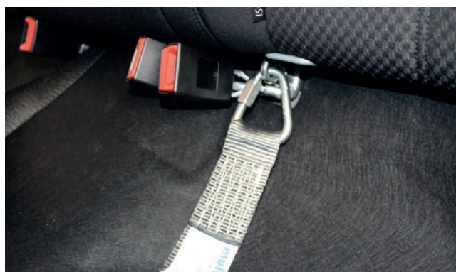
Tether strap fitted to eye bolt
