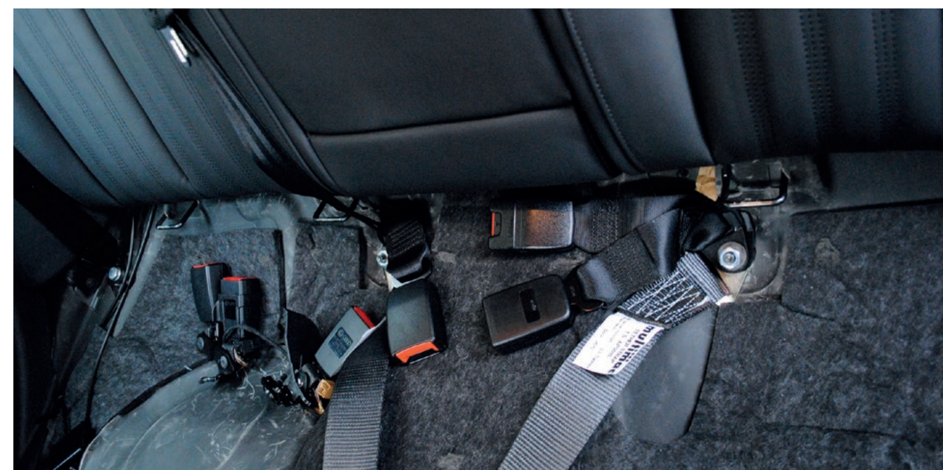
Seat cushion removed showing original [wired] buckles lying loose in the seat well
