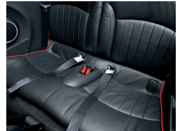
Plastic ISOFIX cover removed to give room for tether strap
