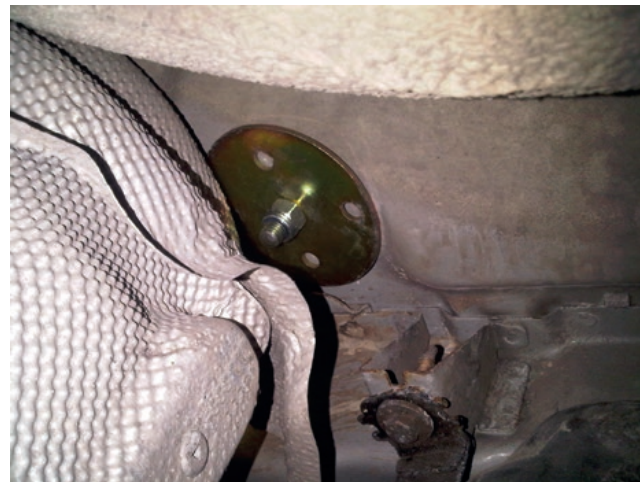
Spreader plates fitted under car floor
