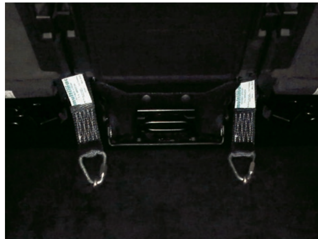
Tether straps fitted to eye bolts
