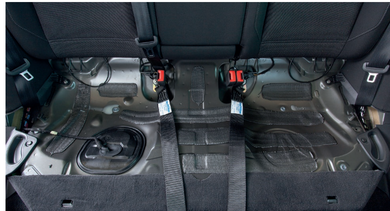
Under the seat cushion, showing the plated tethers fitted
