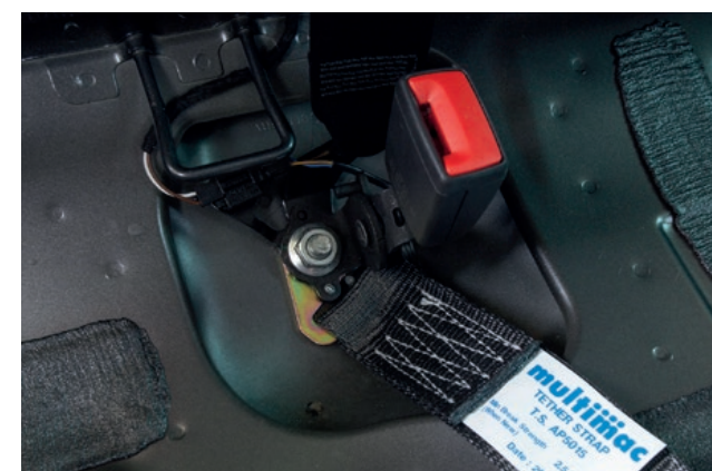
Plated tether fitted above existing buckle, on same stud
