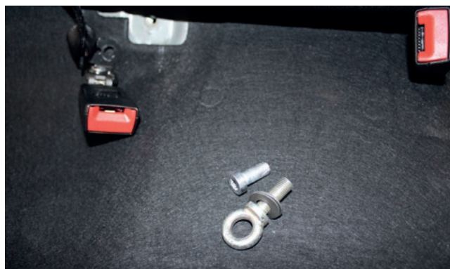
Bolt removed, and Multimac eye bolt
