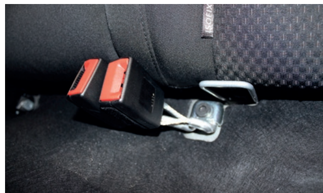
Existing buckles bolted to floor
