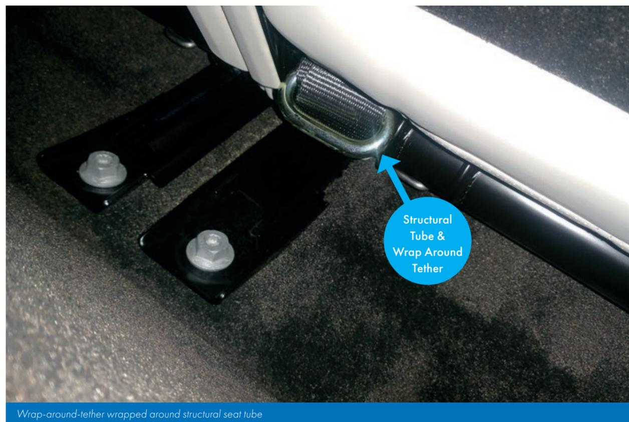
Wrap-around-tether wrapped around structural seat tube
