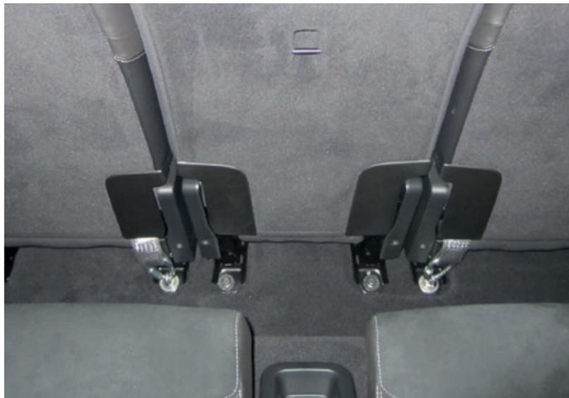
Examples showing eye bolt fixings, and tether strap routings
