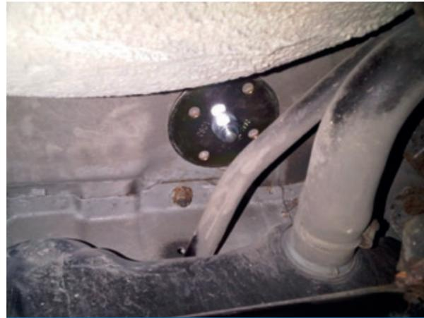
Spreader plates fitted under car floor
