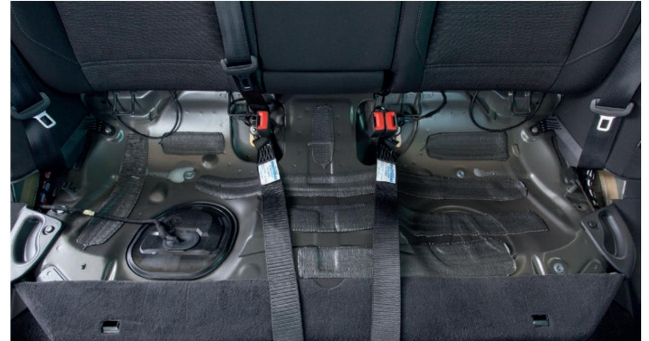
Under the seat cushion, showing the plated tethers fitted
