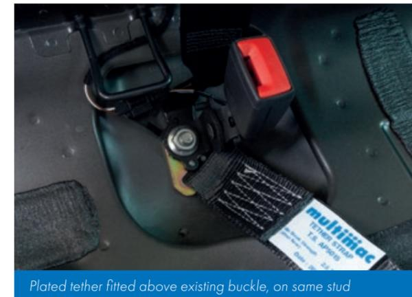
Plated tether fitted above existing buckle, on same stud
