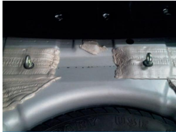
Floor drilled and eye bolts fitted
