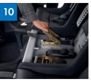
Tighten up both ratchets using the handle. Tighten them up equally rather than 1 before the other, as in some cars this may pull the Multimac to one side.
