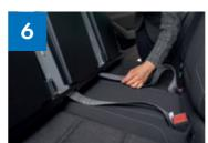
Tilt the Multimac forwards slightly to insert the tether straps through the holes in the back of the chassis.
