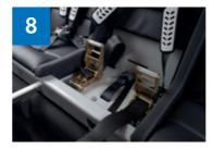
Check that the Multimac is still central in the car. Screw the feet into the legs and slide the legs into the sockets. The final leg length is a matter of trial and error, but if you adjust them so the feet just rest on the floor and measure them to ensure both are the same length, that is a good start. Push them back as far as they will go.
