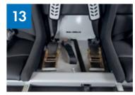
Put the seat cushion/s back in place, making sure the harness is not twisted and comes through the 'recess' at each side of the cushion.
