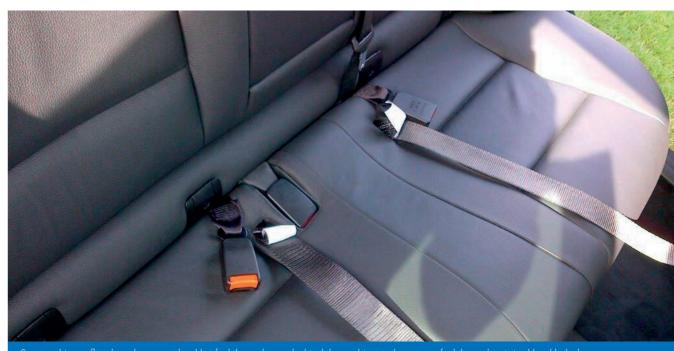
Seat cushion refitted: replacement buckles fed through gap behind the cushion, tether straps fed through original buckle holes
