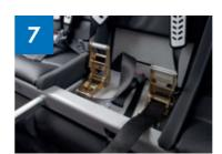
Ensure the straps are not twisted. Feed the tethers through the slot in the spindle. Slide the legs into their sockets.
