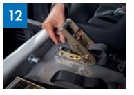
Push any loose tether strap back through the ratchet so it does not hang over the front of the Multimac.
